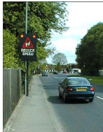
The picture on the left (on Main Road, Biggin Hill) shows a sign warning of an impending dangerous bend (it lights up if the driver is approaching too fast).
