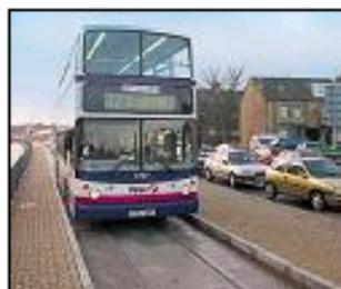
The latter two are likely to be bus based and could be "guided buses" where buses run on a dedicated road and are guided automatically, as shown above. This has proved very successful in Leeds, and they are much cheaper than trams. Other options discussed for the future were trams, and trolley buses.
