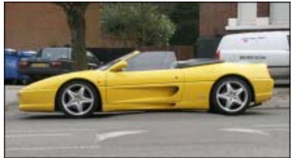
Above is a picture of a Ferrari 355 Spider, parked on a speed cushion on the lower part of Old Hill. As you can see, it grounds on the hump. In fact with a driver and passenger in, it is impossible to cross these humps and caused significant damage when the driver attempted to do so. As he says, a car that adheres to European regulations should not ground on road humps, and in Holland the council would be forced to remove such humps.
