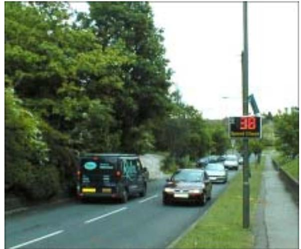
Bromley has been relatively quick to adopt the use of Speed Indicator Devices (SIDs) - above is a picture of a mobile one placed on Leeson Hill. The latest published Road Safety Plan for Bromley contains an interesting analysis of research into their effectiveness.
