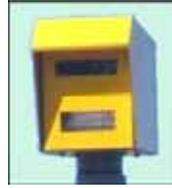
A new type of camera called the "Monitron" is being installed at up to 66 locations in London – see picture left. They are typically positioned at the top of a tall pole. They work by digital photography with images being transmitted via broadband to a central monitoring station, so the whole process can be automated unlike the Gatso devices which require film replacement. Some of these are replacing existing Gatso devices but they are also being installed in new locations.
