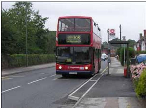
Above is an example of the latest hazard introduced onto Bromley's roads. No not the bus, but the "bus boarder" which is a smaller version of a kerb build-out. This picture was taken in Towncourt Lane, Petts Wood, but proposals for two of these have also been made for Southborough Lane.
