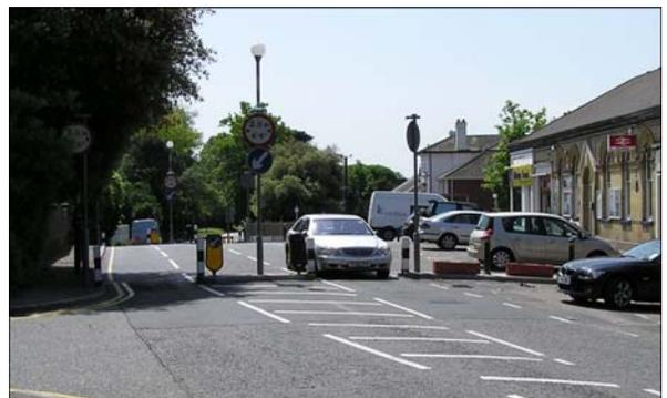
The signs indicate the width restrictions are 6’6” wide but when constructed they were apparently about 6’8”. They have since been widened to about 6’11”. But many cars still cannot get through them without damage.
